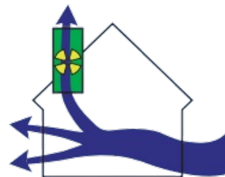
Figure 116: Fan aided natural airflow
