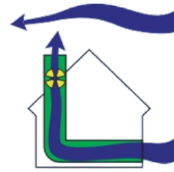
Figure 117: Mechanical ventilation aided by wind and stack
