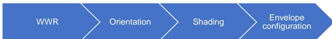
Figure 14 Order of Significance of PCS for Achieving High-Performance Scenario in Affordable Housing: Borey-Type
