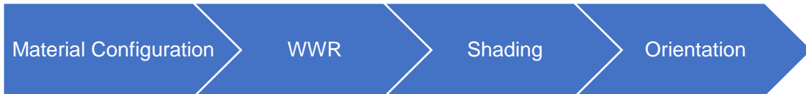
Figure 35 Order of Significance of PCS to Achieve Near-Zero Scenario in MHIH: Borey-Type
