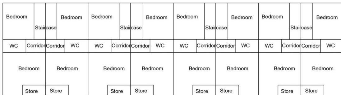
Figure 7 First Floor Plan: Affordable Housing Borey-Type
