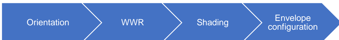
Figure 18 Order of Significance of PCS for Achieving Code Compliance Scenario in Affordable Housing: Borey-Type
